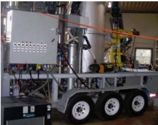
Mobile pyrolysis unit that converts poultry litter to biochar and heating oil; Source: FPPC
